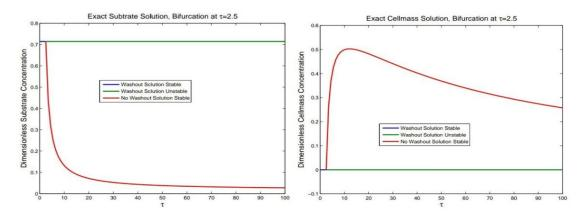
The exact solutions for the dimensionless substrate concentration and cell mass are in the two figures above. The bifurcation that occurs is that the moment the no-washout solution becomesphysical, it also becomes stable, while the no-washout solution then becomes unstable.
